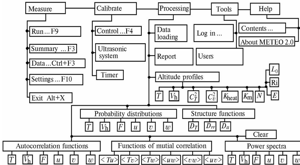
FIG. 2. Menu system of the METEO 2.0 Windows Application.
