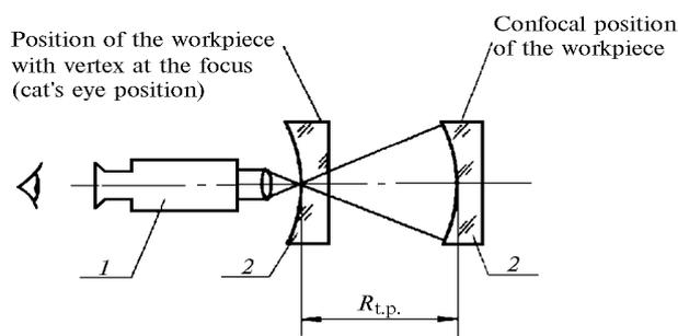
FIG. 1. Geometry of the autocollimation technique to measure the curvature radius: an instrument controlling adjustments (1); a test piece (2).
