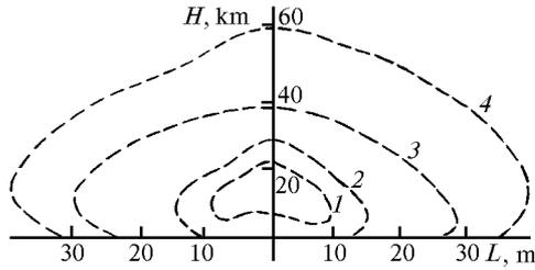
FIG. 1. Shape and dimensions of the zones of active turbulent mixing (aerodynamic wake) perpendicular to the ship longitudinal axis obtained in numerical simulation of a plane ship model at the distance from its bow: 65 (1); 140 (2); 260 (3); and 455 m (4).
