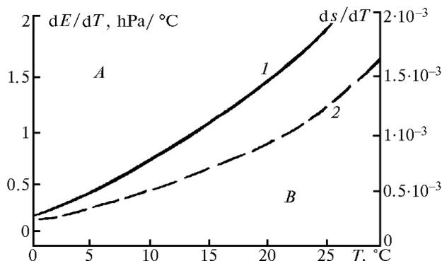
FIG. 2. Formation of cloud tracks behind SS at isobaric mixing of the exhaust gases with air as a function of air temperature and humidity and fuel properties. Zone A – clouds appear, zone B – clouds do not appear,  $dE/dT$  as a function of temperature (curve 1),  $ds/dT$  as a function of temperature (curve 2).
