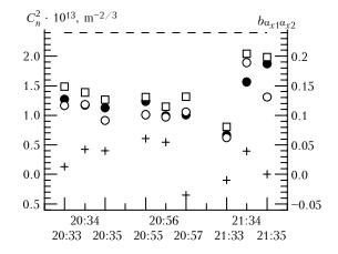
FIG. 2. Comparison of  $C_n^2$  values measured by the single-channel scheme and by the differential technique: differential scheme ( $\Box$ ); simultaneous measurements by meters I and II ( $\bullet$ , ); coefficients of cross correlation between the signals from the I and II meters of the angular displacements of the image (+ – ); the calculated value is shown by the dashed line. Realization length is 40 seconds. The distance between the sub-apertures on the X axis is 68 mm.
