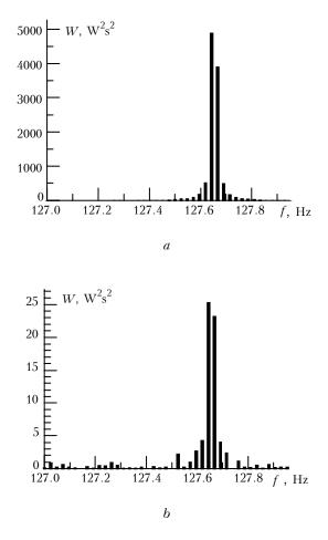
FIG. 3. Power spectra of signals near the fluctuation frequency of the controlled mirror: from the singlechannel meter of the image jitter (a) and from the output of the differential meter (b).
