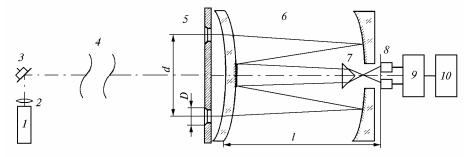
FIG. 1. Block-diagram of the differential meter.
