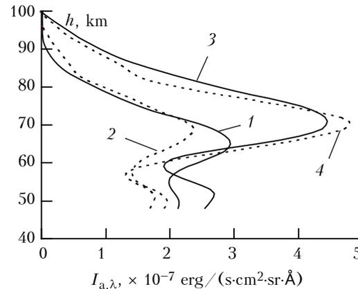
FIG. 2. Altitude behavior of the aerosol component of the spectral brightness of the Earth's atmosphere limb  $I_{a,\lambda}$  in the ultraviolet region ( $\lambda = 273$  and 280 nm).
