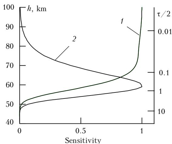
FIG. 4. Sensitivity of the method of tangent sensing at  $\lambda = 280$  nm as a function of the depth of an aerosol scattering layer from the top of the atmosphere related to the coefficient of directional light scattering (1); and to the turbidity coefficient (2).
