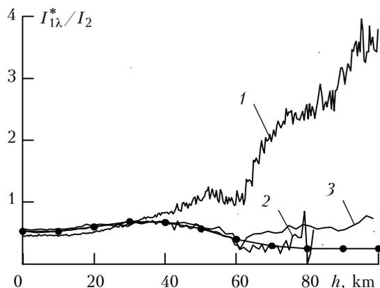
FIG. 1. The ratio,  $I_{1\lambda}^*/I_2$ , of signals in the first and second UV channels of the spectrometer, dots denote the curve showing the contribution from spurious light.
