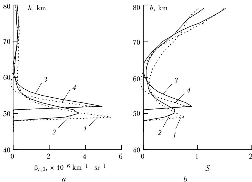
FIG. 3. Altitude behavior of the aerosol scattering characteristics: the coefficient of directional light scattering  $\beta_{a,\theta}$  (a); and the turbidity factor  $S$  at the wavelengths  $\lambda = 273$  and  $280$  nm in the ultraviolet region (b); curves 1–3 present data for midlatitudes and curve 4 for the equatorial zone.
