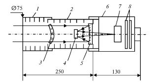
FIG. 3. Optical scheme of the wide-angle sensor: shade with a system of diaphragms (1); Cassegrenian meniscus telescope (2); meniscus (3); secondary mirror (4); primary mirror (5); unit of the photoreceiving device (6): matrix photoreceiving device (7); control board of the matrix photoreceiving device (8).
