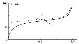
FIG. 1. Altitude dependence of brightness attenuation for the star No. 252 (Ref. 10) at its set behind the Earth's atmosphere: with regard for sensitivity of a specific photoreceiving device (1); for monochromatic radiation at  $\lambda = 255$  nm (2).
