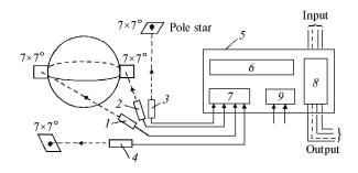
FIG. 4. Block diagram for spacecraft independent navigation and orientation: star field sensors (1 - 4): UV sensors directed to the equator region (1, 2), sensor (UV or visible) directed at the Pole star (3), sensor (UV or visible) with axis parallel to the spacecraft velocity vector (4); electronic unit (5): video processor (6), unit for control over sensors (7), unit for mating with onboard telemetric system of a spacecraft (8); power supply unit (9).
