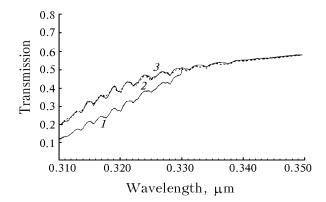
FIG. 1. Calculated values of the atmospheric transmission (solid curves 1 and 3) and experimental data (dashed line 2) obtained at the station "Pik Terskol, B Ref. 2.
