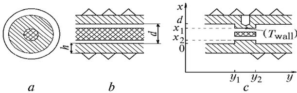
FIG. 1. Discharge chambers: discharge area ; cooled fin surface ; the wall with high thermal conductivity ;  $T$  is the temperature measurement point in the experimental chamber.
