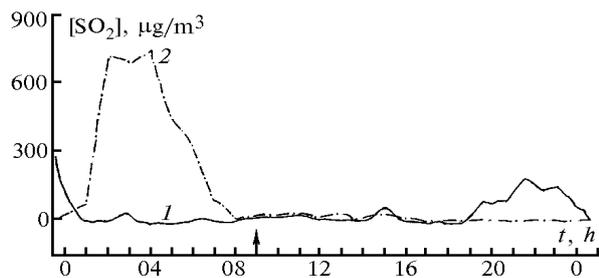
FIG. 3. Diurnal behavior of sulfur dioxide concentration in the surface layer (in the center of Guadalajara City). Curves 1 and 2 are for the measurements on 7th and 9th October, 1995.
