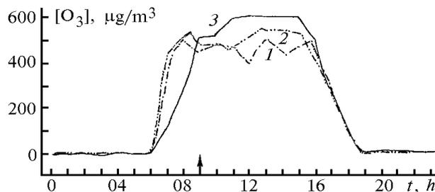
FIG. 2. Diurnal behavior of ozone concentration in the surface layer (in the center of Guadalajara City). Curves 1, 2, and 3 are for the measurements on 7th, 8th, and 9th October, 1995.
