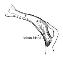
FIG. 4. Water pollution field for the case of gas pipeline break near the left bank.
