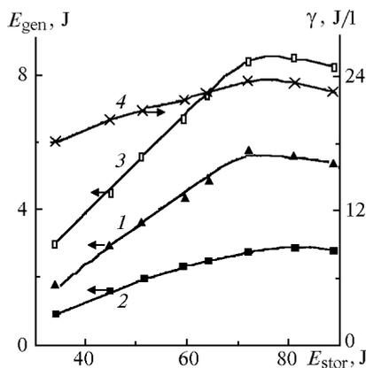
FIG. 4. Energy of generation in the first (1) and second (2) discharge gaps, total output energy of the laser (3), and total specific energy of output laser emission (4) as functions of energy stored in the capacitors of the SMVED power supply. The gas mixture used is  $CO_2:N_2:He = 1:1:3$ , total pressure  $P_{mix} = 0.8$  atm.
