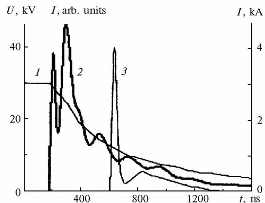
FIG. 3. Oscillograms of the voltage pulses at the second gap (1), discharge current pulses (2), and of the generation pulse (3). The gas mixture used is  $\text{CO}_2:\text{N}_2:\text{He} = 1:1:3$ , total pressure  $P_{\text{mix}} = 0.8$  atm,  $U_{\text{charg}} = \pm 15$  kV.
