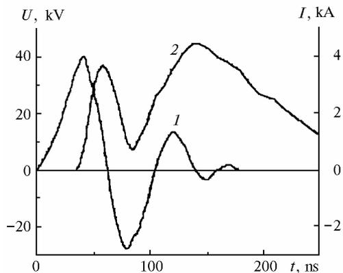
FIG. 2. Oscillograms of the voltage pulses (1) at the central electrode and of the discharge current (2). The gas mixture used is  $\text{CO}_2:\text{N}_2:\text{He} = 1:1:3$ , total pressure  $P_{\text{mix}} = 0.8$  atm,  $U_{\text{charg}} = \pm 15$  kV.
