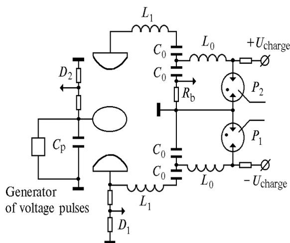
FIG. 1. Block-diagram of the electric circuitry of the installation.  $D_1$  and  $D_2$  are the ohmic voltage dividers;  $R_b$  is the current bypass.
