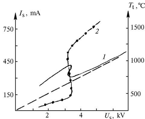
FIG. 2. Volt-ampere characteristic and temperature dependence of GDT and source operation. The GDT parameters are the same as in Fig. 1. The distributed molybdenum electrode in the form of a coil with a resistance of the cold coil of 0.2 Ω was placed inside the GDT. Here,  $f = 3$  kHz, curve 1 is for the VAC of the power supply unit, and curve 2 illustrates the dependence of the active volume temperature of the GDT on  $U_s$ .
