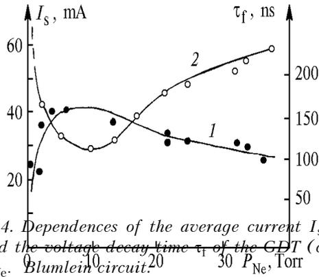
FIG. 4. Dependences of the average current  $I_s$  (curve 1) and the voltage decay time  $\tau_f$  of the GDT (curve 2) on  $P_{Ne}$ . Blumlein circuit.
