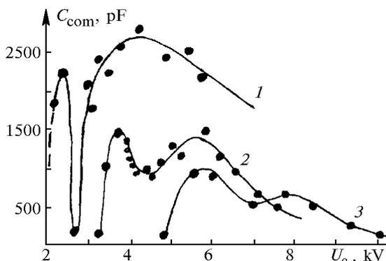
FIG. 1. Dependence of  $C_{com}$  on  $U_c$  for  $f \cong 10$  (1), 5 (2), and 3 kHz (3) calculated from EC (6). The GDT aperture was 20 mm,  $d = 80$  cm,  $P_{Ne} = 200$  Torr for the TGI 1000/25 commutator, and  $C_p = 7920$  pF. The external shunt inductivity  $L_{sh}$  was connected.
