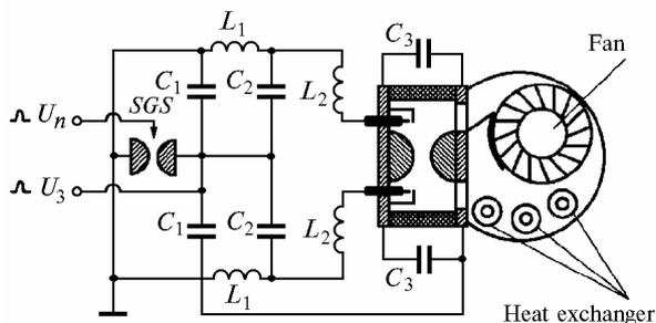
FIG. 1. Circuit diagram and cross section of the laser: SGS denotes the RU-65 spark-gap switch,  $C_1 = 22.5 \text{ nF}$ ;  $C_2 = 45 \text{ nF}$ ;  $C_3 = 17 \text{ nF}$ ;  $L_1 = 2.1 \mu\text{H}$ ;  $L_2$  comprises 39 inductors  $1 \mu\text{H}$  each.
