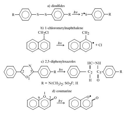
FIG. 1. Scheme of primary stages of photolysis.
