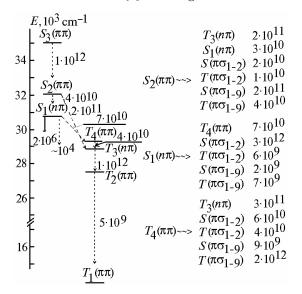
FIG. 5. Electron excited states and scheme of the energy deactivation for  $\alpha$ - and  $\beta$ -breaking of the lactone ring of the coumarine molecule.
