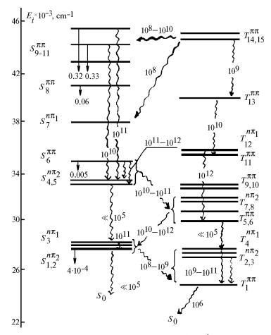
FIG. 4. Scheme of the electron excited states and rate constants (in s<sup>-1</sup>) of the most important nonradiative processes in the TNT molecule.
