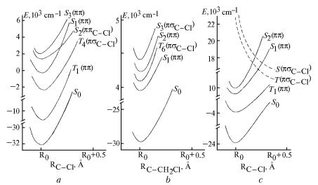
FIG. 3. Potential curves of electron excited states of chlorosubstituted forms of naphthalene in different reaction coordinates: a) I-chloronaphthalene, b and c) I-chloromethylnaphthalene.
