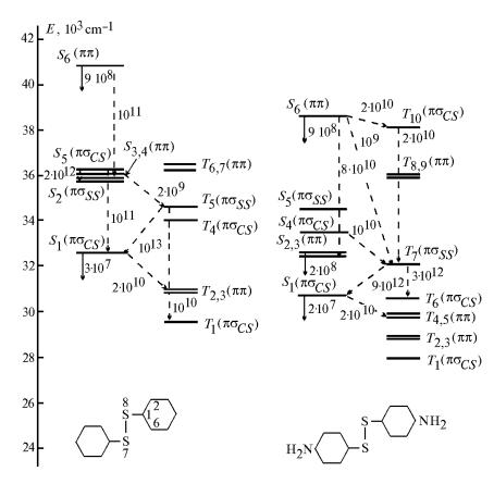
FIG. 2. Scheme of electron excited states and the most effective photophysical processes in the disulfide molecules.
