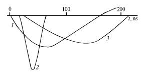
FIG. 1. Waveforms of the discharge current (1) and lasing pulses at  $\lambda = 510.6 \text{ nm}$  (2) and  $\lambda = 780.8 \text{ nm}$  (3).
