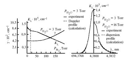
FIG. 4. Measurements of the parameters of the water molecule line at 694.38 nm in nitrogen under nonequilibrium conditions.
