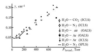
FIG. 5. Broadening of the water molecule line at 694.38 nm by foreign gas pressure measured with different spectrometers.
