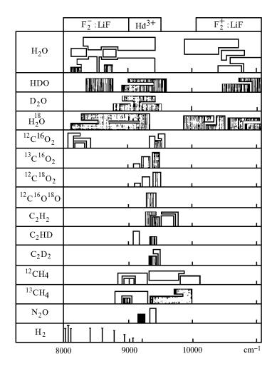
FIG. 3. Molecular absorption bands recorded with the ICLS in the  $8000-11000 \text{ cm}^{-1}$  range<sup>40</sup> (hatched regions indicate the bands recorded first).
