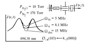
FIG. 10. Transformation of the dip profile of the broadband ruby-laser radiation caused by the 694.38–nm absorption line of the water molecules placed in the dynamic Stark cell.
