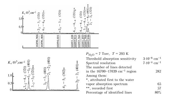
FIG. 1. Water molecule absorption spectrum.
