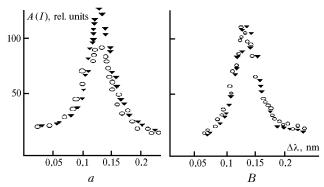
FIG. 7. Spectral dependence<sup>54</sup> of the energy of linearly (a) and circularly (b) polarized ruby-laser radiation absorption in the line at 694.38 nm:  $\blacklozenge$ , I = 5 MW/cm;  $\circlearrowright$ , I = 35 MW/cm.
