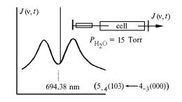
FIG. 9. Signal with a narrow spectrum generated in the dip of broadband ruby-laser radiation formed due to the water molecule absorption line at 694.38 nm.
