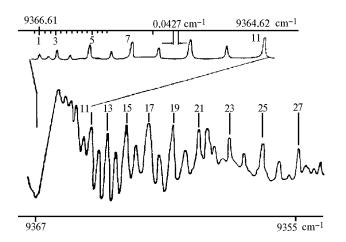
FIG. 2. Absorption spectrum of  $C_2H_2$  molecule recorded with the broadband and narrow-band laser spectrometers.<sup>39</sup>
