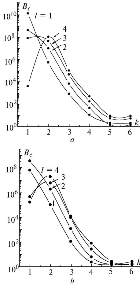
FIG. 1. The coefficient  $B_0$  of overlapping of pumping and SRS fields in an ethanol drop as a function of the input resonance order  $k$  in the case of  $TE_{km}-TE_{l70}$  (a) and  $TM_{km}-TE_{l70}$  (b) generation. The calculation was performed for different output resonance order  $l$ .
