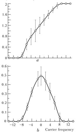
FIG. 1. Estimates of the discrepancies  $\varepsilon_{\varphi}$  (Fig. 1a) and  $\varepsilon_a$  (Fig. 1b) between the phase and the amplitude of a complex function determined in the experiment and calculated using the analytic signal as functions of the carrier frequency. The rms deviations are shown as the confidence intervals.
