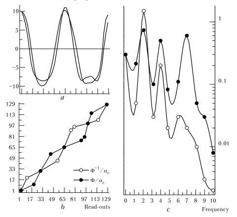
FIG. 3. The extension-compression transformation of a signal with a monotonic phase: the initial signal, (----), and signal after transformation, (---) (a); normalized phase, (----), and normalized inverse phase of the initial signal,  $(-\circ-)$ , (b); the spectrum of the initial signal,  $(-\bullet--)$ , and the spectrum of the transformed signal,  $(-\circ--)$  (c).
