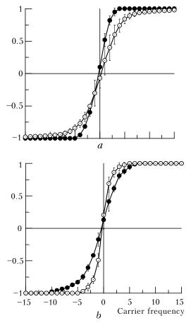
FIG. 2. The estimates of the causality degree  $p_c$ , see open circles (  $-\circ-$  ) and the monotony degree  $p_m$ , see black circle (  $-\bullet-$  ). (a) is the signal with a finite spectrum and amplitude-phase modulation, (b) is the signal with phase modulation. As a confidence intervals we show the rms deviations of the corresponding functions.
