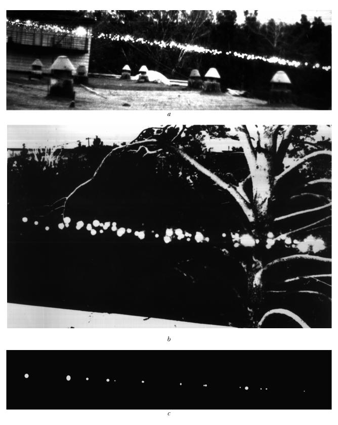
FIG. 2. Panoramic photographs of laser sparks made by focusing of laser radiation at the distance F = 120 m into the atmosphere. The focal spot area was S = 10 (a, b) and  $3 \text{ cm}^2$  (c). The laser energy density in the laser beam caustic was Q = 18 (a), 8 (b), and 6 J/cm<sup>2</sup>(c). The objective field-of-view angle of the Zenit camera was  $34.5^{\circ}$ .
