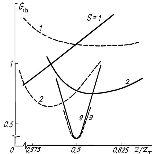
FIG. 3. Threshold gain for the cophased (dashed curves) and antiphased (solid curves) mode vs. the distance to coupling mirror  $z$  for different orders of diffraction coupling  $S$ .  $N = 10$  and  $a/\sigma = 12$ .
