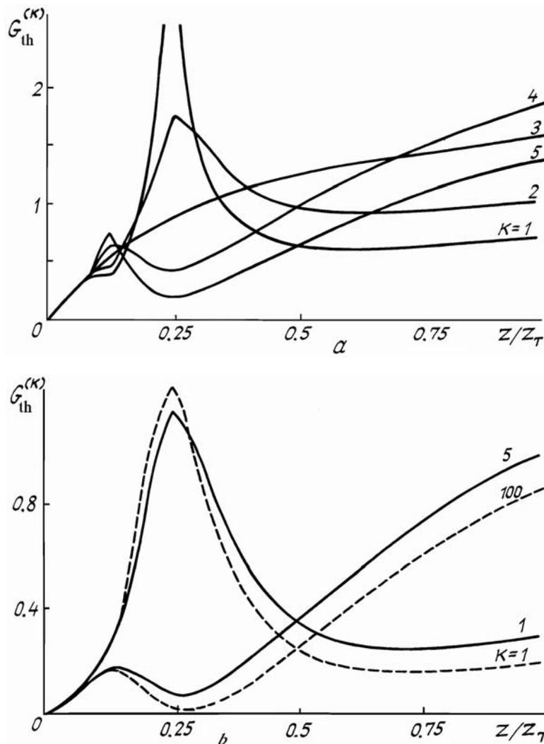
FIG. 2. Threshold gains for collective modes  $G_{th}^{(k)}$  vs. distance  $z$  to the coupling mirror ( $\kappa$  is the number of a mode): a)  $a/\sigma = 6$  and  $N = 5$ ; b)  $a/\sigma = 4$  and  $N = 5$  (solid curve) and  $N = 100$  (dashed curve).
