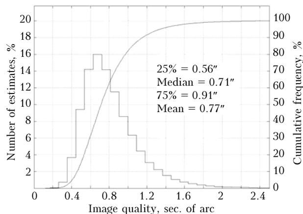
**Fig. 2.** Statistics of the image quality. The ordinate axis is on the right of the histogram and the cumulative distribution is on the left.
