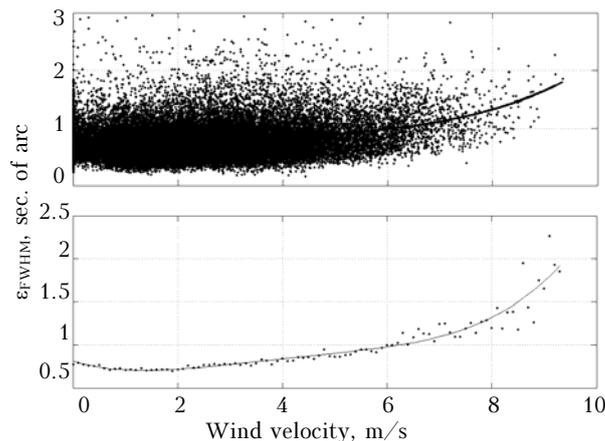
**Fig. 3.** The  $\epsilon_{FWHM}$  as a function of wind velocity at the Mt. Maidanak for the period from May 2000 until October 2002. The bottom plot is made by averaging image quality values corresponding to the wind velocity range  $\Delta V = 0.1$  m/s.
