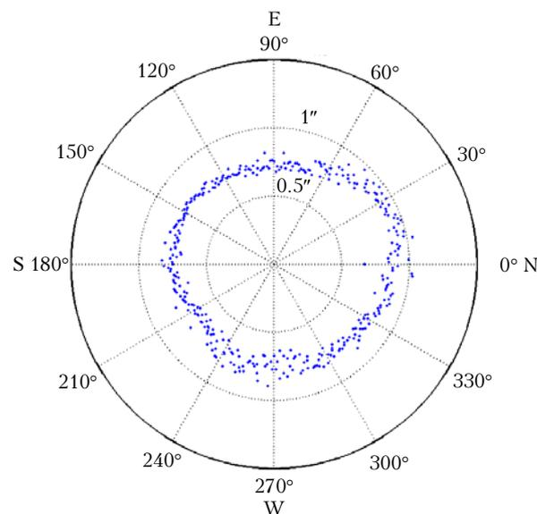
**Fig. 4.** Image quality as a function of ground wind direction; deterioration is pronounced at northers.
