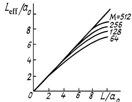
FIG. 1. Effective outer scale of turbulence as functions of the number of the nodes of computational grid and of the ratio  $L/a_0$ .
