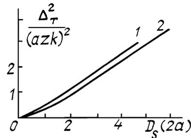
FIG. 2. Turbulent broadening as a function the structural phase function of the spherical wave: 1) analytical estimate and 2) method of numerical simulation.
