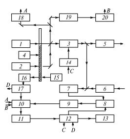
FIG. 1. Experimental prototype of lidar: He-Ne lasers (1 and 2); an electrooptic modulator (3); a chopper (4); a collimator (5); a telescope (6); a PbSe photoresistor (7); a spectrum analyzer (8); a detector (9); a multiplexor (10); an analog—to—digital converter (11); a microcomputer (12); a display (13); a LFM generator (14); a light diode (15); a Ge photodiode (16); a synchronizer (17); pirodetectors (18 and 20); and,  $CH_4$  cell (19).
