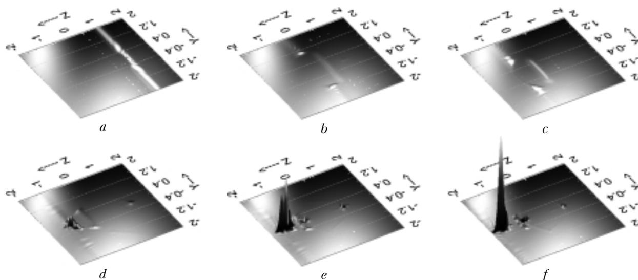
**Fig. 1.** Spatial distribution of the relative optical field intensity in the plane of the principal cross section of a water droplet with  $a_0 = 20 \mu\text{m}$  exposed to a plane wave with the following parameters:  $\lambda = 0.8 \mu\text{m}$ ,  $t_p = 50 \text{ fs}$ ,  $t_0 = 100 \text{ fs}$  at different time  $t = 70$  (a), 130 (b), 170 (c), 200 (d), 220 (e), and 250 fs (f). The oval in white shows the particle boundary. The radiation propagates from right to left.
