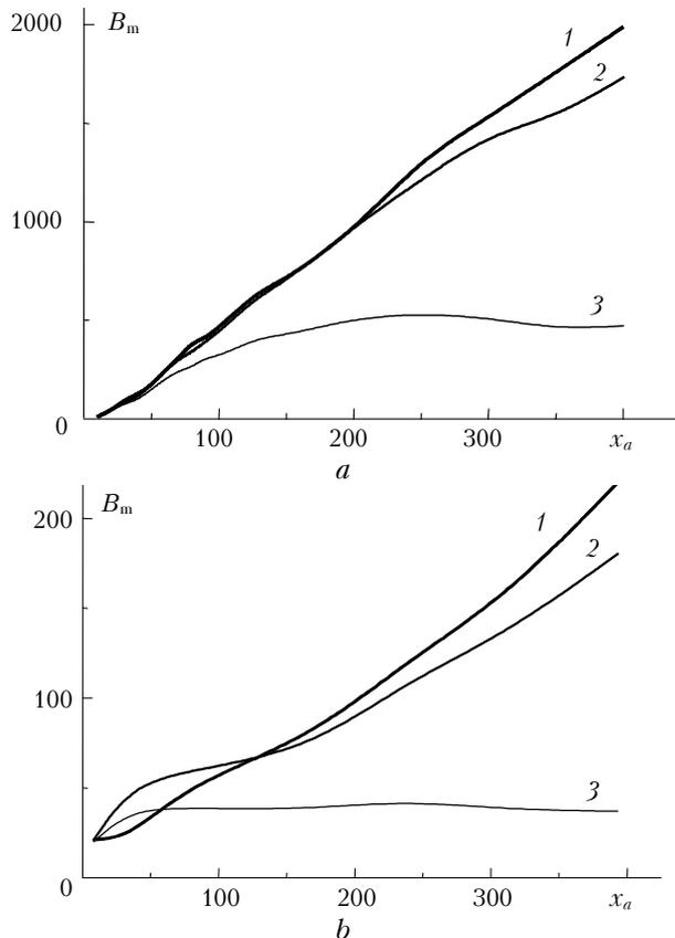
**Fig. 3.** Dependence of the maximum values of the optical field inhomogeneity factor  $B_m$  in the zone of geometrical focus behind the particle ( $a$ ) and at the rear maximum inside the particle ( $b$ ) on the diffraction parameter  $x_a = 2\pi a_0/\lambda_0$  at different level of absorption:  $\kappa_0 = 10^{-8}$  (1),  $10^{-4}$  (2),  $10^{-3}$  (3).
