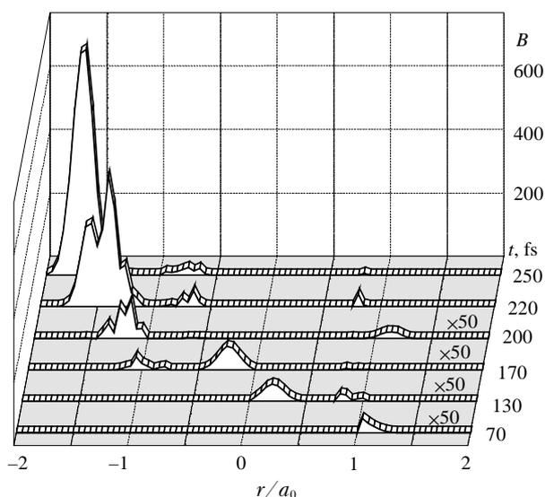
**Fig. 2.** Distribution of the relative intensity of the optical field along the principal diameter of a water droplet with  $a_0 = 20 \mu\text{m}$  exposed to a plane wave. The radiation parameters are the same as in Fig. 1. The intensity at the first four curves is increased by 50 times.
