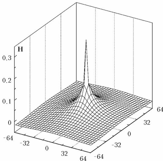
Fig. 2. Pulsed response function of 128 × 128 size.
