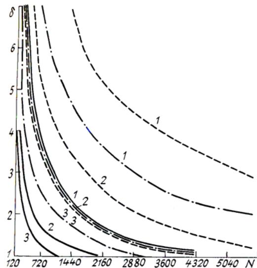
FIG. 1. Minimum relative deviation  $\delta = (M_a - M_n)/M_n$  of the anomalous Na concentration as a function of the number of soundings  $N$ , detected with prescribed efficiency
