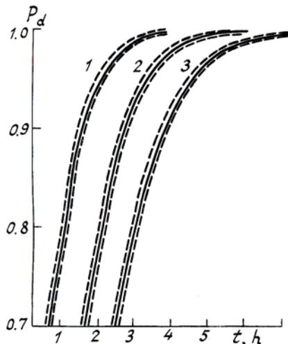
FIG. 3. Attainable probability of detection  $P_d$  of the sporadic layer (—) and its boundaries (---) as functions of the sounding time  $t$  for  $\alpha = 10^{-1}$  (1),  $10^{-2}$  (2),  $10^{-3}$  (3).
