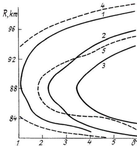
FIG. 2. The required sounding height  $R$  as a function of  $\delta$  for detecting (—) with  $\alpha = 10^{-1}$   $P_d = 0.9$  (1);  $\alpha = 10^{-2}$   $P_d = 0.99$  (2);  $\alpha = 10^{-3}$   $P_d = 0.999$  (3), and measuring the anomalous concentration  $M_a$  (---) with  $\delta_\mu = 0.4$  (4), 0.2 (5) for  $N = 4320$ .
