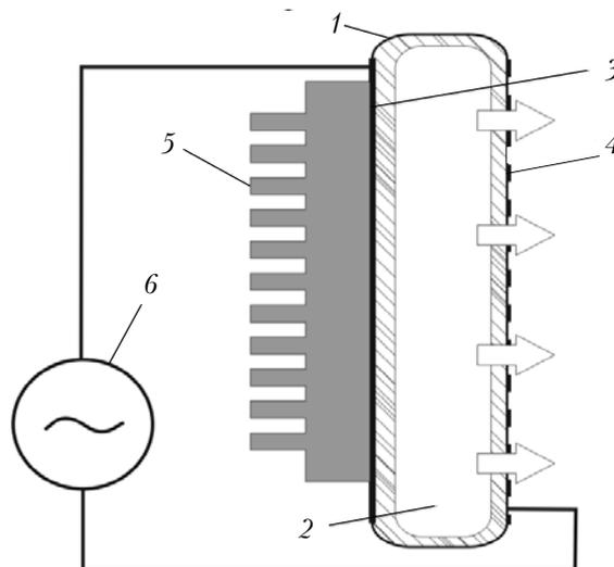
**Fig. 1.** Setup construction: planar flask (1); gas-discharge volume (2); solid reflecting electrode (3); perforated electrode (4); radiator (5); pulse energy source (6). The arrows indicate the direction of radiation output.
