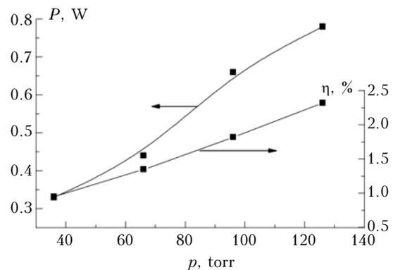
Fig. 2. The dependence of excilamp radiation average power and efficiency in  $Xe-Br_2 = 400-1$  gas mix on the pressure of inertial gas.
