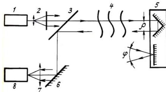
FIG. 2. Block diagram of the experimental arrangement: 1 - LG-38 laser; 2 - collimator; 3 - beam-splitting plate; 4 - layer of nonuniform medium; 5 - reflectors; 6 - mirror; 7 - receiving objective; 8 - tracking unit.
