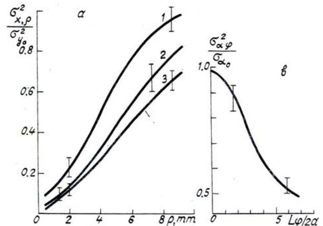
FIG. 3. The displacement of the lidar image of the source versus the separation of the axes with reflection from a prism (a) and with reflection from a flat mirror (b).
