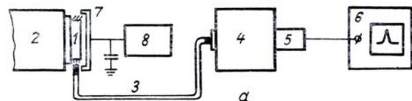
FIG. 1a. Block diagram of the experimental setup: 1) active element; 2) electron beam; 3) optical waveguide; 4) spectral device; 5) PMT; 6) oscilloscope; 7) Faraday cylinder; 8) voltmeter.
