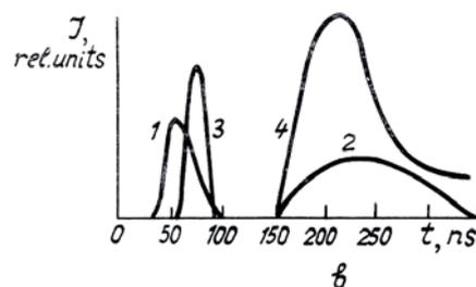
FIG. 1b. Oscillograms of current pulses produced by electron beams with energy 190 (1) and 600 keV (3), and of the corresponding laser radiation pulses (curves 2 and 4).
