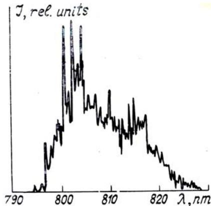
FIG. 2. Spectrum of the  $Ti^{3+}$ :  $Al_2O_3$  laser emission at an energy of the pumping electron beam of 190 keV.
