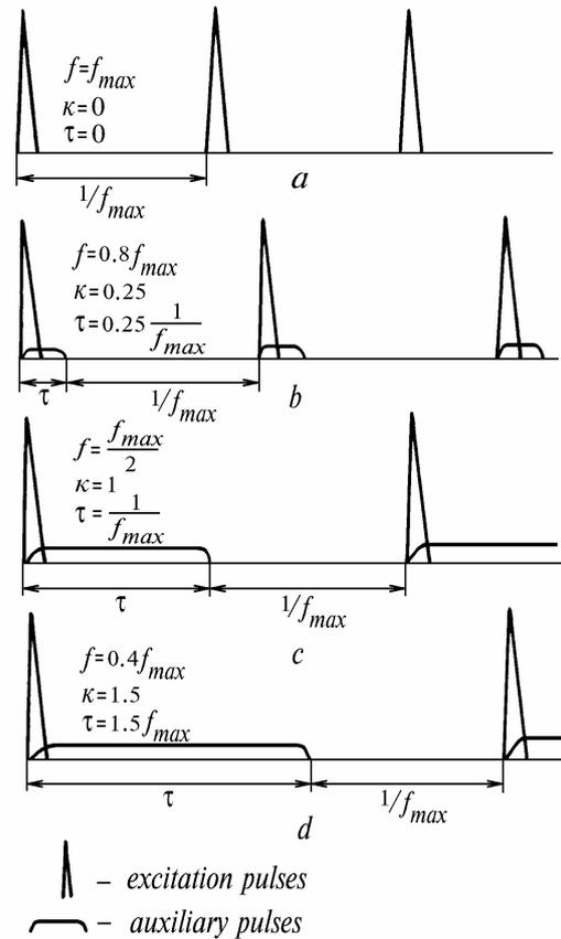
FIG. 1. Diagrams of the method of laser excitation with stabilization of output energy on varying  $f$ .
