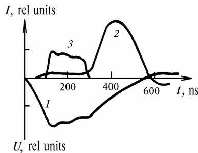
FIG. 7. Waveforms of voltage (1), current (2), and laser radiation (3) for the mode of controlled ionization.
