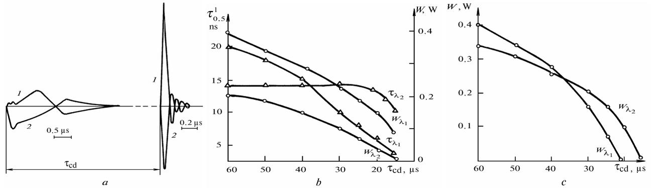
FIG. 3. Typical waveforms of current (1) and voltage (2) of the control pulses (on the left) and excitation pulses (on the right) (a). Dependence of the duration and average output power (b, c) for the green (1) and yellow (2) spectral lutes on the time delay  $\tau_{cd}$ .
