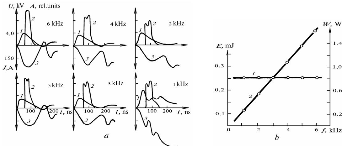
FIG. 2. Waveforms of voltage (1), laser radiation (2), current (3) (a) as  $weU$  as the pulse energy (1) and average power (2) (b) as functions of pulse repetition rate for a laser operating in the stabilization mode..
