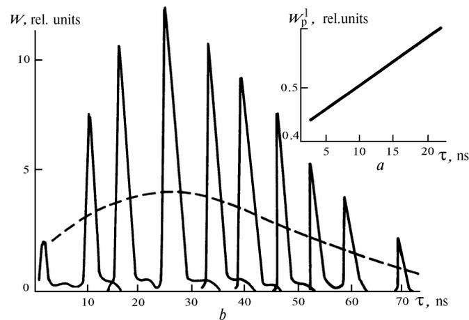
FIG. 5. Dependence of  $W$  of the OA system on  $\tau^1$  (a). Pulsed power  $W_p^1$  of the OA system oscillator i excitation pulses of the oscillator and amplifier (b). Dashed curve indicates superemission.
