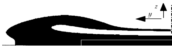
Fig. 3. Region of starting points, starting from which the particles fall into the sampler ( Stk = 0.4 , W = 2 m/s, h = 0.01 m).
