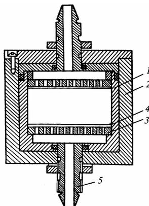
FIG. 3. Regeneration filter for the active medium.
