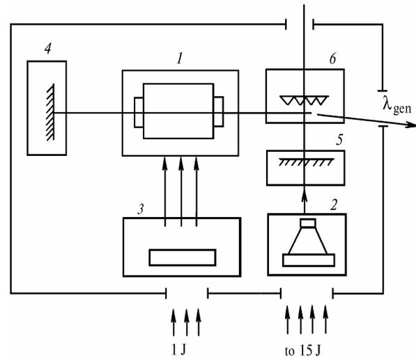
FIG. 1. Block-diagram of the "MZhL-01" powerful dye laser: 1) cell with dye solution, 2) cell-cone, 3) cylindrical lens, 4 and 5) mirrors, and 6) diffraction grating.
