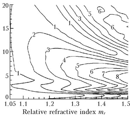
**Fig. 1.** Maximum relative error (%) of the extinction coefficients in pairs among equivalent ensembles of randomly oriented ellipsoidal particles (1), (2) and the equivalent polydisperse ensemble of spherical particles with the power-law distribution as a function of the maximum diffraction parameter  $kc$  at different relative refractive indices of the particulate matter.
