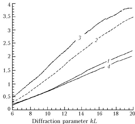
**Fig. 3.** The extinction efficiency factor of randomly oriented ice hexagonal cylinders ( $L/d = 6$ ) calculated using the FDTD method (1), equivalent (2) and equisurface (3) spherical particles<sup>4</sup> and by means of the equivalent ensemble of spherical particles (4).
