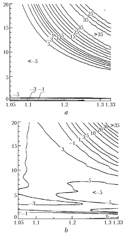
**Fig. 2.** Relative error  $\Delta$  (%) in calculating the extinction coefficients of the ensemble of randomly oriented oblate ( $\epsilon = 2$ , *a*) and elongated ( $\epsilon = 0.5$ , *b*) round cylinders by means of the equivalent ensemble of spherical particles as a function of the relative refractive index  $m_r$  and the maximum diffraction parameter  $\rho_{\max}$ ;  $\epsilon$  is the ratio of the base diameter to the length of the cylinder.
