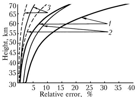
FIG. 1. Vertical profiles of the error in measuring air density by means of lidars with the parameters corresponding to the BALKAN-3 lidar (1); pulse energy is increased up to 0.5 J (2); the accumulation time is also increased up to 20 sec (3). Solid curves are for space version of the lidars, and dashed curves are for the ground-based lidars.
