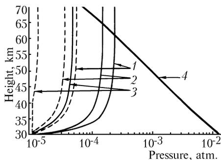
FIG. 2. Absolute error in reconstructing the profile of pressure (4) from data obtained with the lidars whose parameters are the same as in Fig. 1. Solid curves are for space version of the lidars, and dashed curves are for the ground-based lidars.
