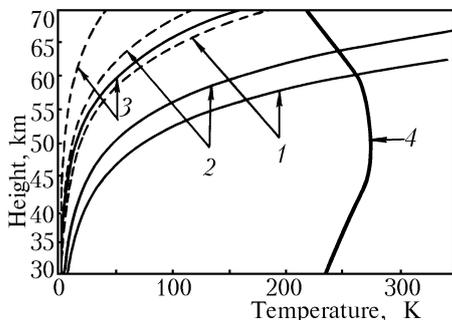
FIG. 3. Absolute error in reconstructing the profile of temperature (4) by means of the lidars whose parameters are the same as in Fig. 1. Solid curves are for spaceborne lidars, and dashed curves are for ground-based lidars.
