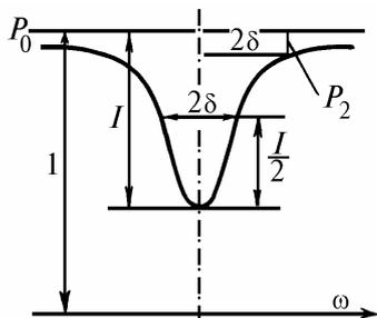
FIG. 1. Dip in the ICL spectrum.
