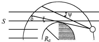
FIG. 1. Scheme of sounding of the twilight Earth's atmosphere. The Sun, the Earth center, and a device lie in the same plane.
