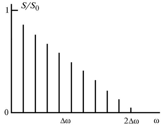
FIG. 1. The spectrum of the narrow-band noise envelope at the output of narrow-band system with  $\Pi$ -shaped AFC.
