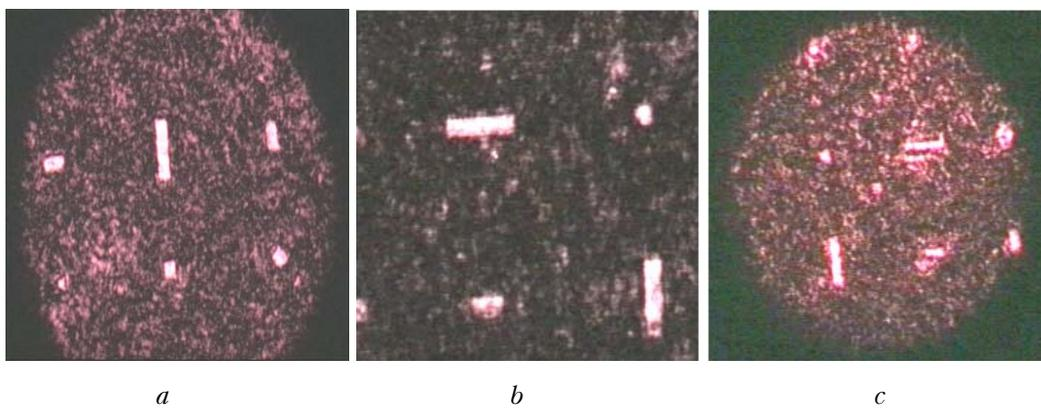
**Fig. 4.** Reconstructed holographic images of model objects.
