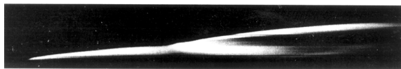
Fig. 1. Streak photograph of a plasma torch that arose under the effect of two laser pulses with the second pulse delayed by 8 \mu\text{s} with respect to the leading edge of the first pulse.
