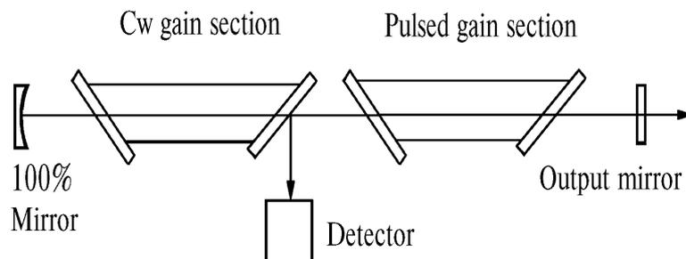
FIG. 1. Schematic diagram of the hybrid autodyne lidar.
