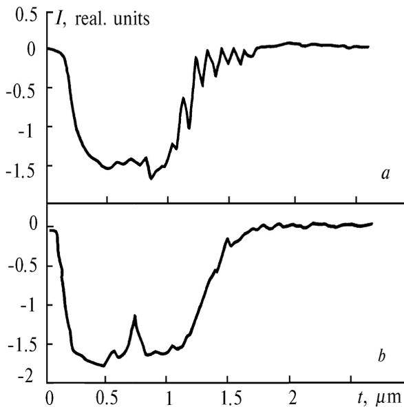
FIG. 3. Typical laser shapes of the output pulse with external feedback: for attenuation using 0 (a) and 30 dB (b).
