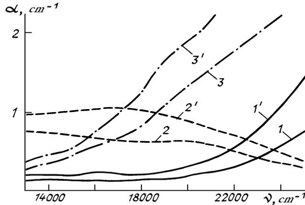
FIG. 4. Extinction coefficients of the layer of suspension of the BS-4 glass particles. The thickness of the layer was equal to 0.1 and 1 cm.  $n_D = 1.52$  (1 and 1'), 1.51 (2 and 2'), 1.53 (3 and 3'), 1, 2, 3)  $d = 0.1$  cm; 1', 2', 3')  $d = 1$  cm.
