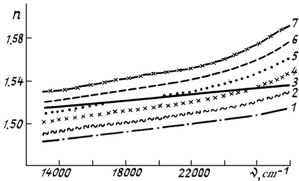
FIG. 1. Dispersion of the refractive indexes of the BS-4 glass (curve 1) and immersion liquids with  $n_D = 1.49$  (2), 1.50 (3), 1.51 (4), 1.52 (5), 1.53 (6), and 1.54 (7).
