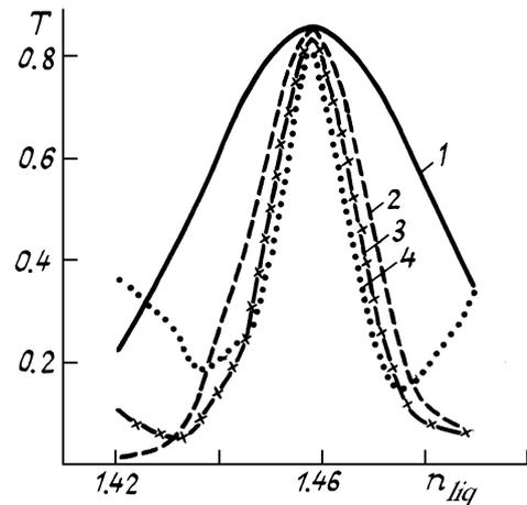
FIG. 5. Transmission of the layer of suspension of particles dispersed in immersion liquids ( $\nu = 1700$   $\text{cm}^{-1}$ ,  $d = 5$  mm) for the particles with radii  $a = 1$  (1), 5 (2), 10 (3), and 15 (4) mm. Dots denote the results of calculations.
