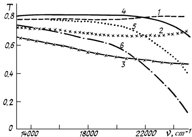
FIG. 6. Transmission of the layer of suspension of the BS-4 glass particles of radius 1 mm dispersed in immersion liquid with  $n = 1.49$  (1), 1.52 (2), 1.51 (3), 1.52 (4), 1.53 (5), 1.54 (6). The thickness of the layer was 1 mm. Dots denote the results of calculations.
