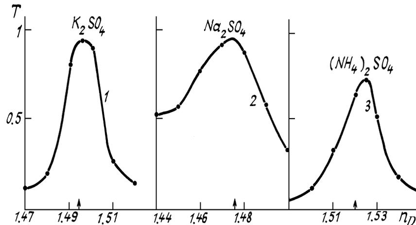
FIG. 2. Experimental curves of the transmission of the layer of suspension ( $d = 5$  mm) as functions of the refractive index of immersion liquid: 1)  $K_2SO_4$ ; 2)  $Na_2SO_4$ ; 3)  $(NH_4)_2SO_4$ .
