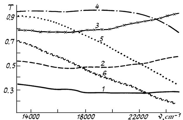
FIG. 3. Transmission spectrum (experiment) of the BS-4 glass particles dispersed in immersion liquids with  $n_D = 1.49$  (1), 1.50 (2), 1.51 (3), 1.52 (4), 1.53 (5), and 1.54 (6).
