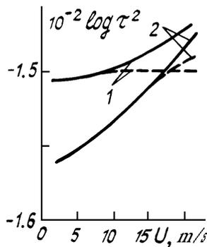
FIG. 2. Duration of echo-pulse received from the sea surfacet trough the clear atmosphere.
