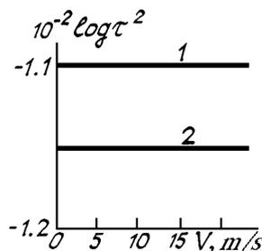
FIG. 3 Duration of echo-pulse received from the sea surface through the dense aerosol atmosphere.
