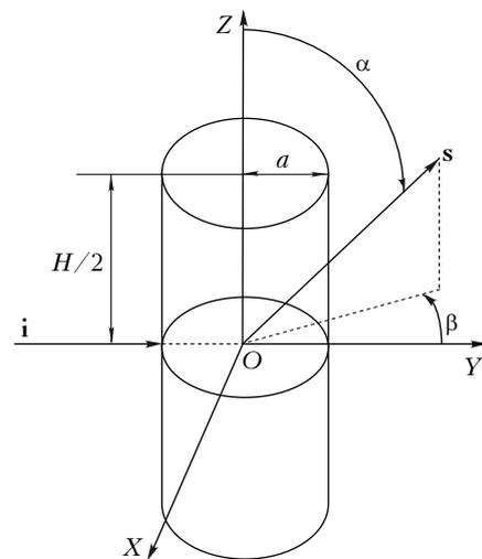
**Fig. 1.** Geometry of light scattering by a circular cylinder of  $a$  in radius and  $H$  in height ( $i$  and  $s$  are unit vectors of incident and scattered light, respectively).
