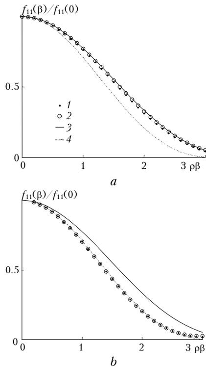
**Fig. 2.** Normalized small-angle light scattering phase function  $f_{11}(\beta)/f_{11}(0)$  as a function of  $\rho\beta$  for an infinitely long (1) and finite-length circular cylinders in WKB (2) and RGD (3) approximations and for the Fraunhofer diffraction (4) at the refraction index  $m = 1.03$  and phase shifts  $\Delta = 0.72$  (a) and  $\Delta = 90$  (b).
