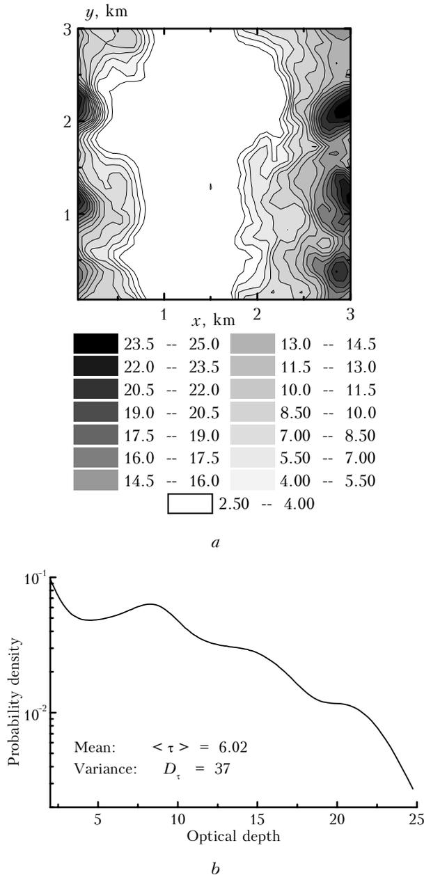
FIG. 1. Two-dimensional field (a) and probability density (b) of the optical depth.
