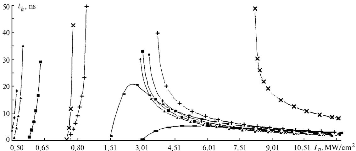
Fig. 1. Duration  $t_k$  of the quasistationary lasing of POPOP solution in ethanol vs. pump power for different pump wavelength at  $L = 0.2$  cm,  $r_1 = r_2 = 0.8$ ,  $n = 5 \cdot 10^{16}$  cm<sup>-3</sup>: 350 (—), 360 (—♦—), 365 (—▲—), 375 (—+—), 380 (—×—), 385 (—■—), and 390 nm (—■—).
