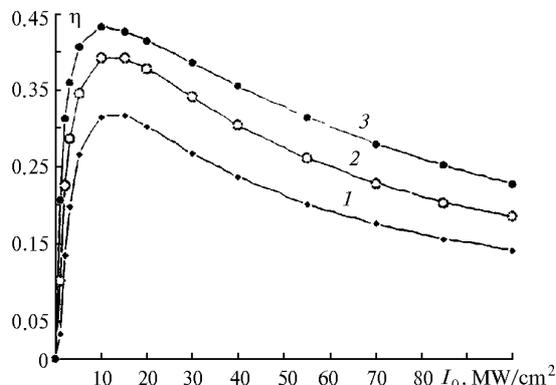
Fig. 2. Lasing efficiency  $\eta$  of POPOP in ethanol vs. pump intensity at different reflection coefficients  $r$ .
