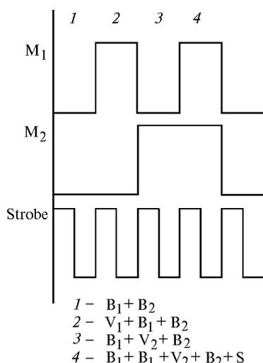
**Fig. 2.** The diagram of operation of the modulators and strobe to obtain a signal.
