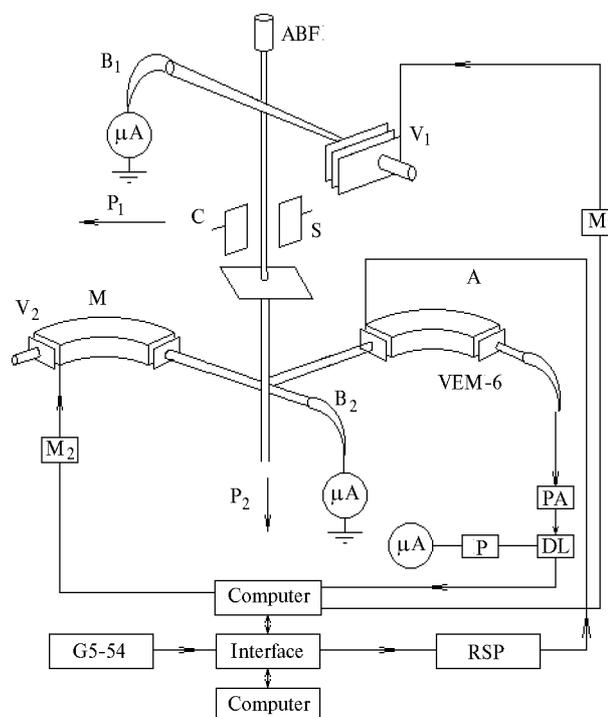
**Fig. 1.** Block-diagram of the experimental setup.
