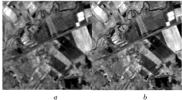
Fig. 7. Fragment of the image retrieved by inversion of the PSF (a) and the corresponding fragment of the initial image (b).
