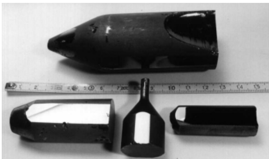
Fig. 4. ZnGeP 2 crystals grown by the vertical Bridgman method on seeds with different orientation: [116], [132], [102], and [100].
