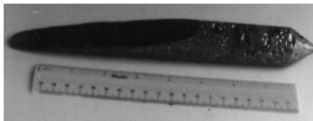
Fig. 3. Polycrystal bar of ZnGeP 2 synthesized at the IOM, feed mass of 415 g.
