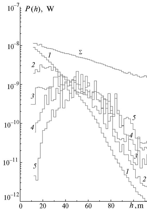
FIG. 5. Dependence of  $P(h)$  and distribution over the orders of multiple scattering calculated for a cloud with high optical density and parabolic shape of the extinction coefficient profile. Curves 1-5 show the order of multiple scattering,  $\Sigma$  corresponds to  $P(h)$ .
