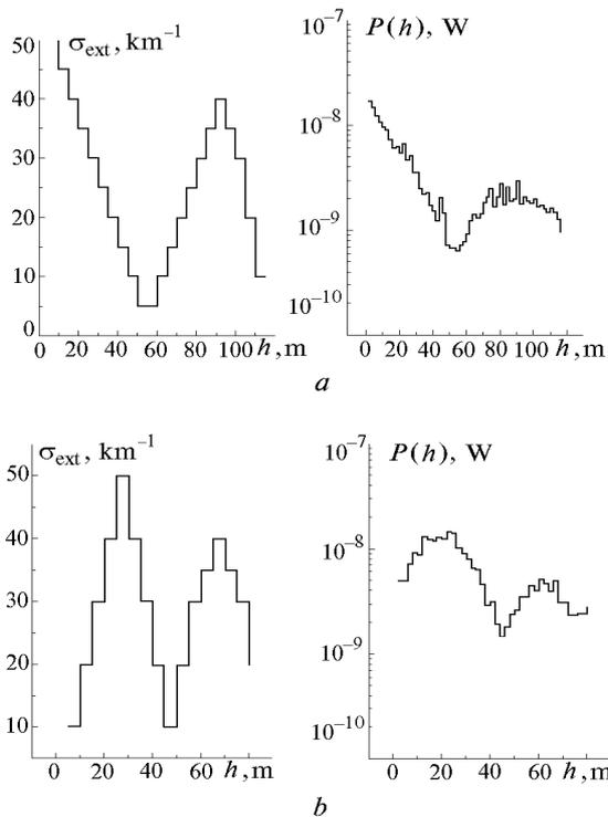
FIG. 3. The return signal power  $P(h)$  for the shape of  $\sigma_{\text{ext}}(h)$  profile with several maxima.
