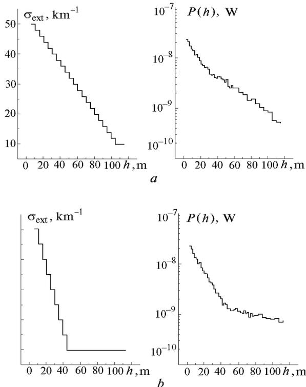
FIG. 1. Lidar return  $P(h)$  as a function of the extinction coefficient profile  $\sigma_{\text{ext}}(h)$ .
